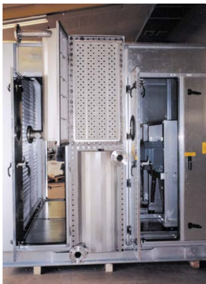
Water/Gas Heat Exchanger
